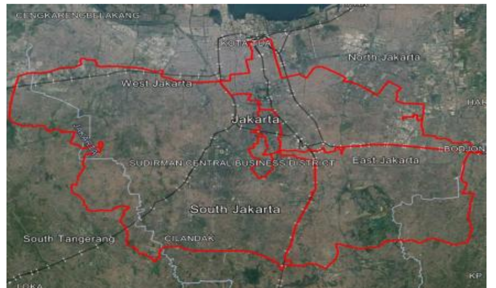
Figure 10. Inner Jakarta Fiber Backbone (458 Km)
