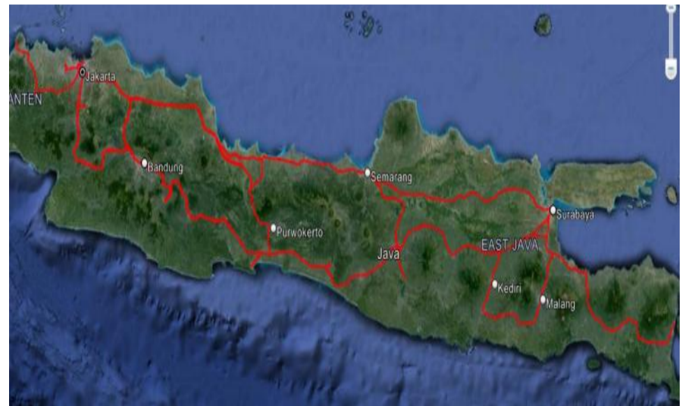
Figure 8. Railway Fiber Backbone (5017 Km)
